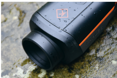
Objective focusing is beneficial for I.D. but rarely immediately critical to initial detection if set around 100m
