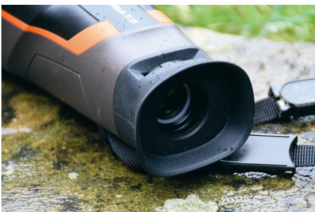
Note the ocular lens focus wheel for internal screen clarity. In use, the OLED screen showed superb optical clarity
